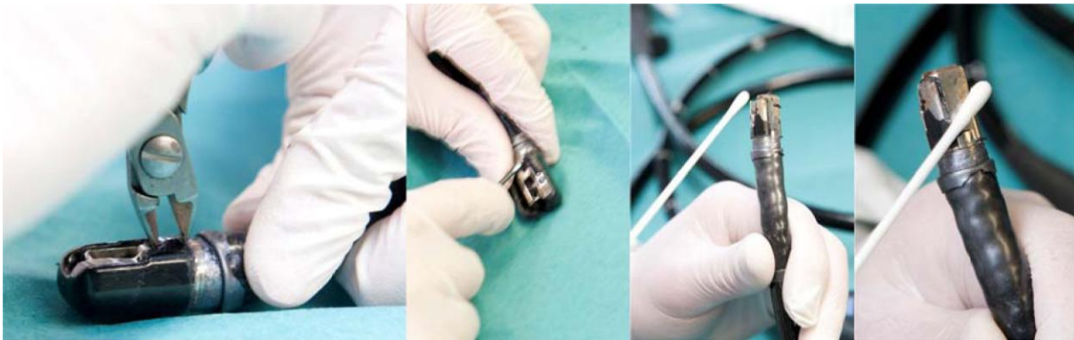
Figure 9: (First two photos on the left) Cutting open and prying loose of the hard plastic cap on the tip. (Two photos on the right) Sampling interior under the removed hard plastic cap.
