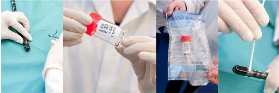
Figure 8: Removing and packaging of the sealant between the hard plastic cap of the tip and the cardan rubber of the scope and (far right) sampling under the cardan rubber.
